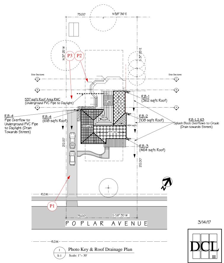
Total Roof Drainage Rain Barrel Capture = 1,552 sqft
